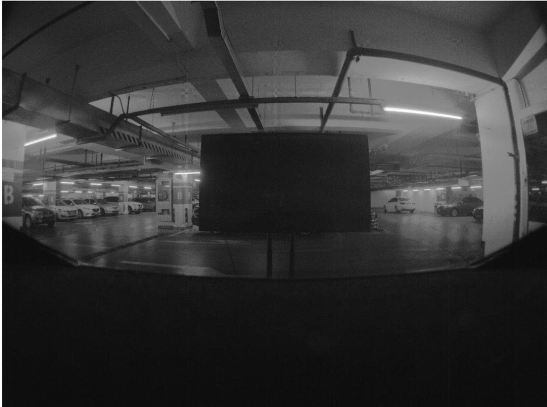
Fig 23. The image captured by the fisheye camera, and we played our adversarial image on the display. (the distortion of the fisheye camera causes the proportion of the area occupied by the display in the image to be greatly reduced)
