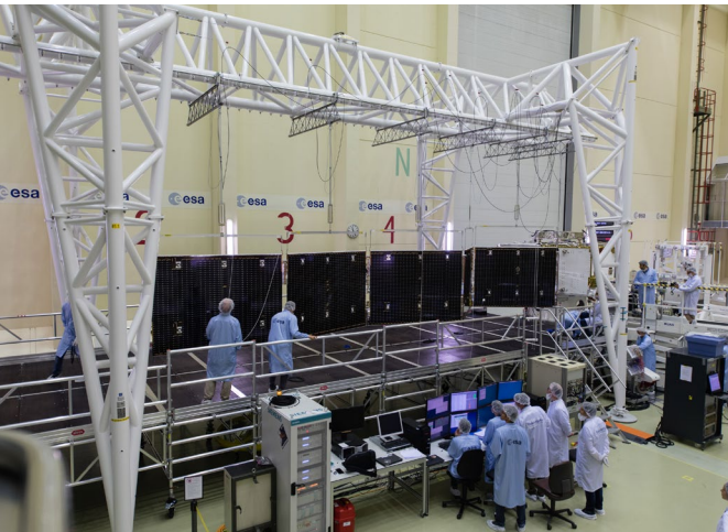
MERCURY TRANSFER MODULE SOLAR WING DEPLOYMENT
